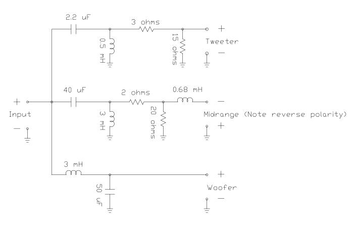
Positive driver terminals are marked with a red dot. Capacitors must be non-polar types with a voltage rating of 50 V or more (preferably 100 V). Capacitors may be paralleled to achieve specified values. Inductors should be air core. Do not mount inductors in top of each other. Resistors should be 10 Watts of more.
