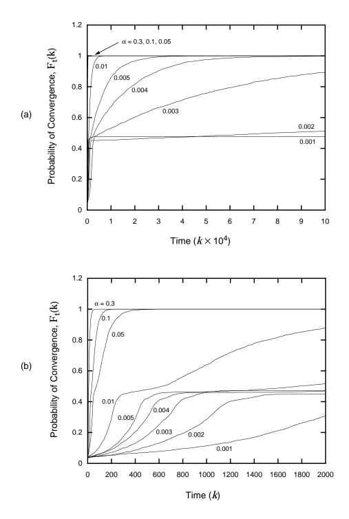
**Fig. 3-2.** The fraction of trials that converge within *k* symbols is plotted versus the number of symbols for a noiseless first-order DD PLL with 16-QAM input alphabet and various step sizes: (a) the number of symbols ranges from 0 to 100,000; (b) an expanded view of the first 2000 symbols.
