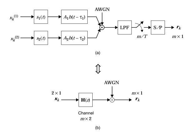
Fig. 5-5. Models for a two-user asynchronous CDMA application: (a) continuoustime model with a chip-rate receiver; (b) equivalent discrete-time model.
