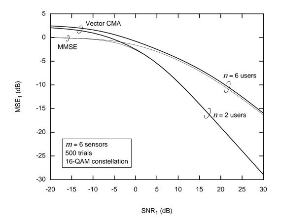
Fig. 4-4. A comparison of the mean-squared error versus SNR of the vector CMA detector and the minimum-MSE detector.
