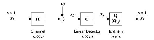
Fig. 4-5. A block diagram of a memoryless channel followed by a memoryless linear detector and a memoryless unitary rotator.
