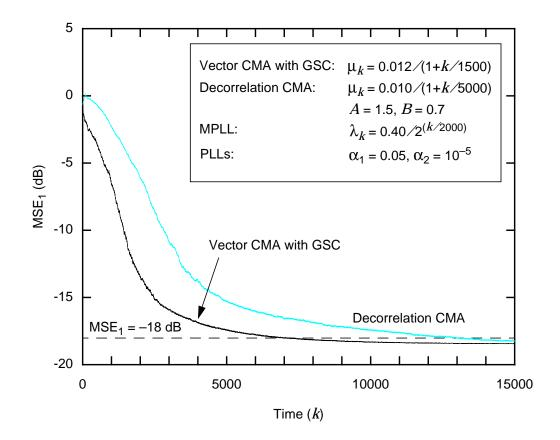
Fig. 5-4. Comparison of the vector CMA with GSC detector and decorrelation CMA detector, in terms of  $\text{MSE}_1$  versus time, for a  $2\times 2$  uniform linear with multipath.
