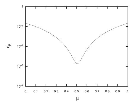
Fig. 3-11. The squared error between the two intermediate points  $\textit{\textbf{v}}_{\lambda}$  and  $\textit{\textbf{v}}_{\mu}$  as a function of  $\mu.$
