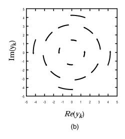
**Fig. 2-5.** If the ambiguity in the input signal to the PLL is a constant phase offset, then the received constellation will be a tilted version of the transmitted constellation as shown in (a). The o's represent the transmitted 16-QAM constellation and the x's represent the received constellation. If the ambiguity is a constant frequency offset, the received constellation will spin, as illustrated in (b).
