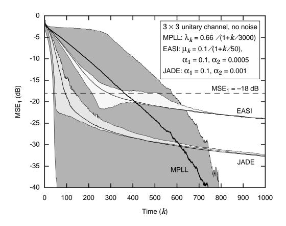
Fig. 3-23. Comparison of the MPLL, JADE, and EASI, in terms of MSE<sub>1</sub> versus time, for a  $3 \times 3$  noiseless unitary channel. The shaded regions represent the variation in convergence time for each of the detector. For each detector, the lower curve is an average of the fastest 10% of the trials, the middle represents the average MSE, and the upper curve is an average of the slowest 10% of the trials.
