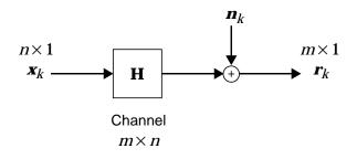
**Fig. 4-1.** A block diagram of an  $m \times n$  noisy memoryless channel model.
