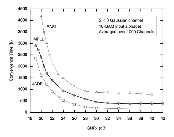
**Fig. 3-28.** The convergence time for each detector is plotted versus SNR<sub>1</sub> for a  $5 \times 3$  noisy complex Gaussian channel followed by a  $3 \times 5$  ideal whitener and a 16-QAM input alphabet. The optimal parameters for each detector can be found in Table 3-5.
