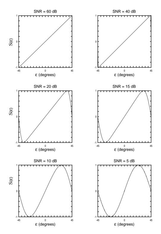
**Fig. 3-3.** Normalized S-curves for a first-order DD PLL with 4-QAM input alphabet and a noisy input signal.
