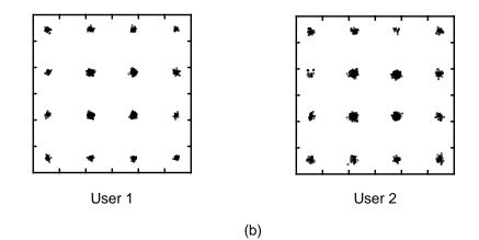
Fig. 4-12. The vector CMA detector applied to a uniform linear-array with halfwavelength spacing and a shaped 16-QAM input alphabet: (a) learning curves, assuming both an actual MPLL and an MMSE MPLL; (b) constellations from the last trial, baud 9000 to 10,000.
