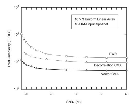
Fig. 4-8. Comparison of the total complexity of the three detector versus SNR<sub>1</sub> for a 16  $\times$  3 uniform linear-array with half-wavelength spacing application with 16-QAM input alphabet. The optimal parameters for each detector can be found in Table 4-1.
