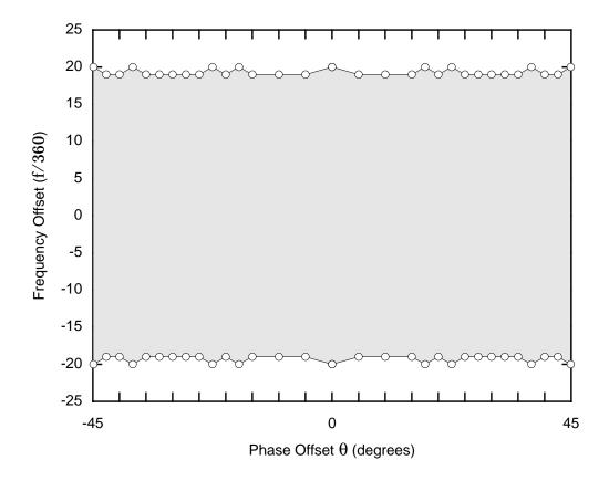
Fig. 3-6. A phase-plane portrait for a second-order DD PLL with parameters  $\alpha_1 = 0.1$  and  $\alpha_2 = 10^{-3}$ .
