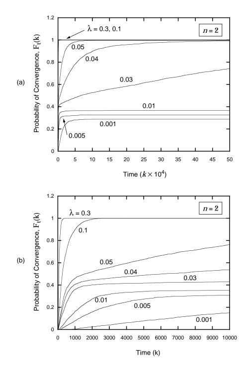
**Fig. 3-14.** The fraction of trials that converge within k symbols is plotted versus the number of symbols for a noiseless two-user first-order MPLL with 16-QAM input alphabet and various step sizes: (a) the number of symbols ranges from 0 to 500,000; (b) an expanded view of the first 10,000 symbols.
