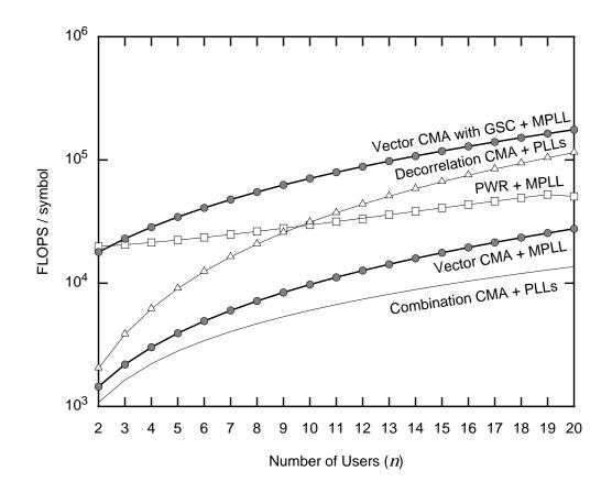
**Fig. 4-13.** Comparison of the computational complexity of the various detectors versus the number of users n for a fixed number of sensors m = 20.
