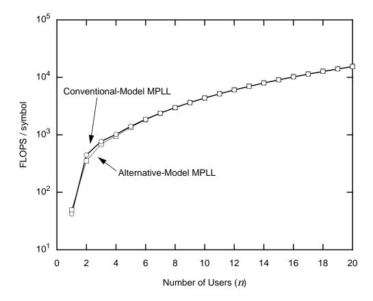
Fig. 3-13. Comparison of computational complexity for the conventional-model MPLL and the alternative-model MPLL.
