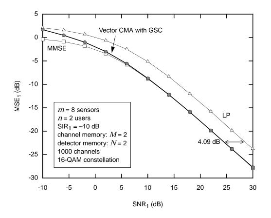
Fig. 5-3. A comparison of the mean-squared error versus SNR of the optimal vector CMA with GSC detector, the optimal minimum-MSE detector, and optimal forward-backward LP detector.
