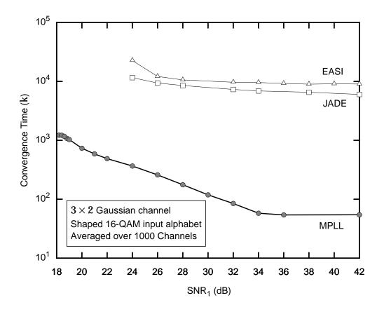
**Fig. 3-27.** The convergence time for each detector is plotted versus  $SNR_1$  for a  $3 \times 2$  noisy complex Gaussian channel followed by a  $2 \times 3$  ideal whitener and a shaped 16-QAM input alphabet. The optimal parameters for each detector can be found in Table 3-4.
