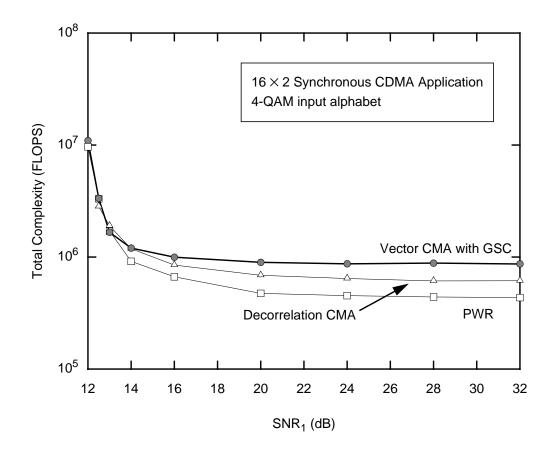
**Fig. 4-11.** Comparison of the total complexity of the three detector versus SNR<sub>1</sub> for a synchronous CDMA application. The optimal parameters for each detector can be found in Table 4-2.
