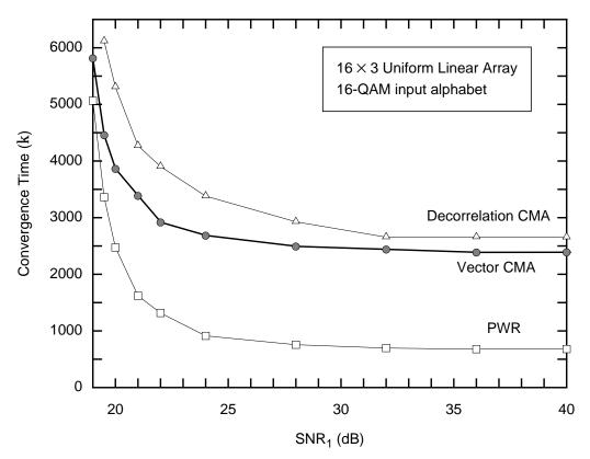
Fig. 4-7. Comparison of the convergence time of the three detector versus SNR<sub>1</sub> for a  $16 \times 3$  uniform linear-array with half-wavelength spacing application with 16-QAM input alphabet. The optimal parameters for each detector can be found in Table 4-1.
