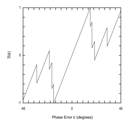
Fig. 3-1. A normalized S-curve for a first-order DD PLL with 16-QAM input alphabet.
