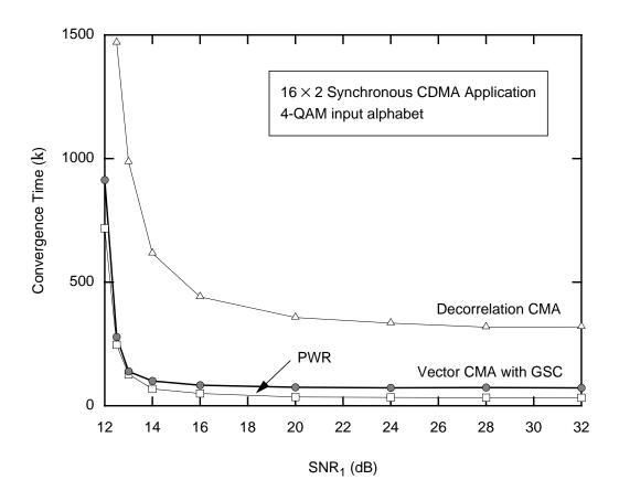
**Fig. 4-10.** Comparison of the convergence time of the three detector versus SNR<sub>1</sub> for a synchronous CDMA application. The optimal parameters for each detector can be found in Table 4-2.
