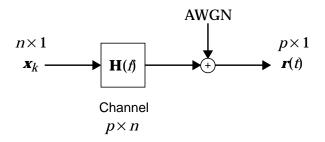
**Fig. 2-1.** A block diagram of a complex baseband  $p \times n$  continuous-time channel model.
