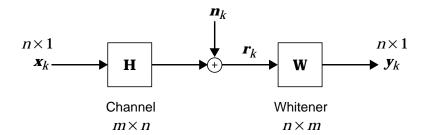
**Fig. 3-20.** A block diagram of an  $m \times n$  memoryless channel followed by an  $n \times m$  ideal whitener. This model is used to generate the input signal for all computer simulations.
