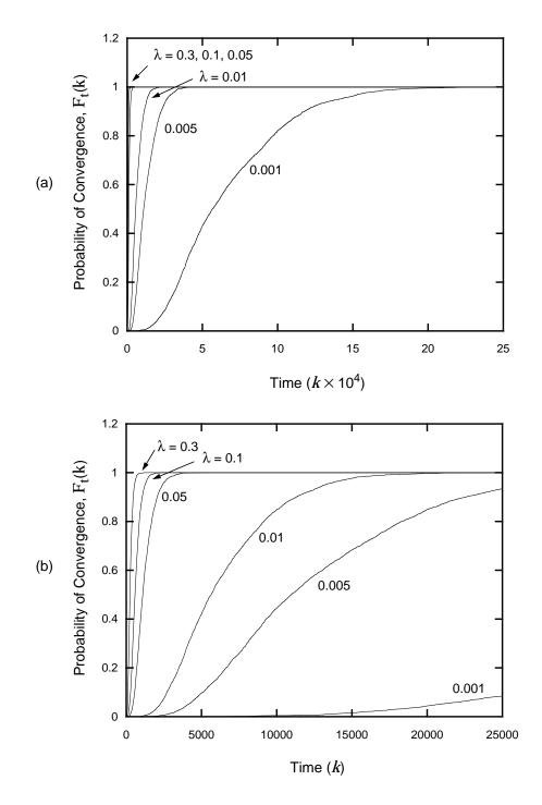
**Fig. 3-18.** The fraction of trials that converge within *k* symbols is plotted versus the number of symbols for a noisy three-user first-order MPLL with 16-QAM input alphabet, various step sizes, and  $SNR_1 = 20 \text{ dB}$ : (a) the number of symbols ranges from 0 to 250,000; (b) an expanded view of the first 25,000 symbols.
