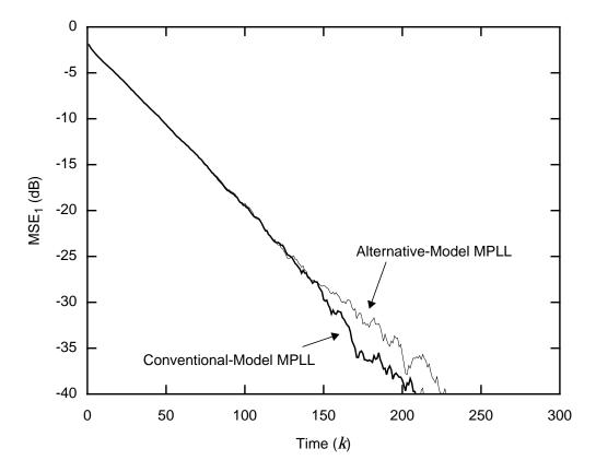
Fig. 3-12. Comparison of the conventional-model MPLL and the alternative-model MPLL in terms of MSE<sub>1</sub> versus time.
