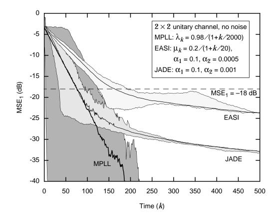
Fig. 3-21. Comparison of the MPLL, JADE, and EASI, in terms of MSE<sub>1</sub> versus time, for a  $2 \times 2$  noiseless unitary channel. The shaded regions represent the variation in convergence time for each of the detector. For each detector, the lower curve is an average of the fastest 10% of the trials, the middle represents the average MSE, and the upper curve is an average of the slowest 10% of the trials.
