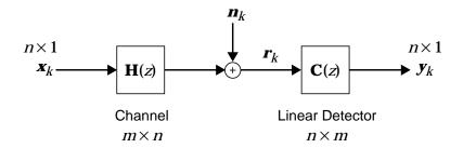
**Fig. 2-3.** A block diagram of an  $m \times n$  channel with followed by an  $n \times m$  linear detector with memory.
