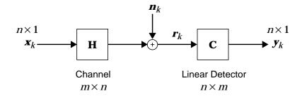
**Fig. 4-2.** A block diagram of an  $m \times n$  memoryless channel followed by an  $n \times m$  memoryless linear detector.
