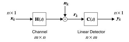
**Fig. 5-2.** A block diagram of an  $m \times n$  channel with followed by an  $n \times m$  linear detector with memory.
