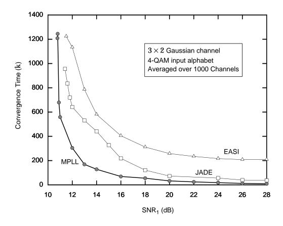
**Fig. 3-25.** The convergence time for each detector is plotted versus  $SNR_1$  for a  $3 \times 2$  noisy complex Gaussian channel followed by a  $2 \times 3$  ideal whitener and a 4-QAM input alphabet. The optimal parameters for each detector can be found in Table 3-2.
