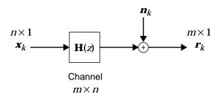
**Fig. 5-1.** A block diagram of an  $m \times n$  noisy channel with memory.
