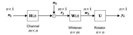
Fig. 1-1. A block of the general whiten-rotate structure.
