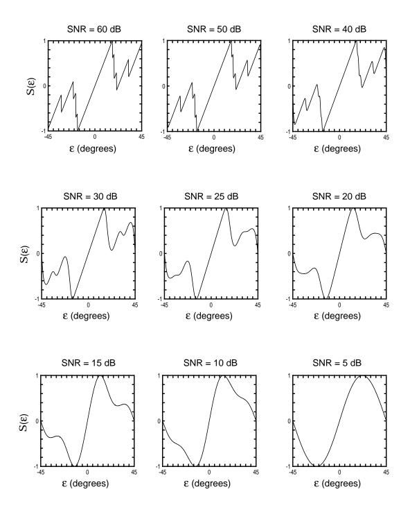
Fig. 3-4. Normalized S-curves for a first-order DD PLL with 16-QAM input alphabet and a noisy input signal.
