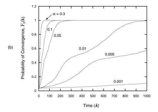
**Fig. 3-5.** The fraction of trials that converge within *k* symbols is plotted versus the number of symbols for a noisy first-order DD PLL with 16-QAM input alphabet and various step sizes: (a) the number of symbols ranges from 0 to 10,000; (b) an expanded view of the first 1000 symbols.
