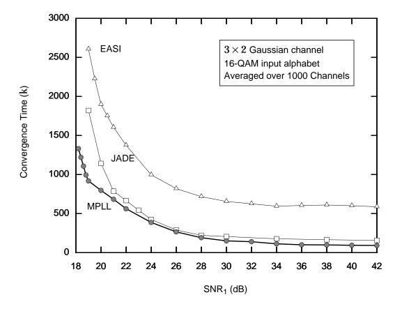
**Fig. 3-26.** The convergence time for each detector is plotted versus  $SNR_1$  for a  $3 \times 2$  noisy complex Gaussian channel followed by a  $2 \times 3$  ideal whitener and a 16-QAM input alphabet. The optimal parameters for each detector can be found in Table 3-3.
